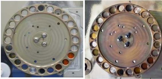
**Fig. 7 Images of the spectrometer materials taken at the start and end of the in-orbit phase of the mission.**
