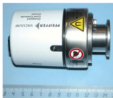
Fig. 3 As-bought cold cathode pressure gauge, showing the original casing and magnet
