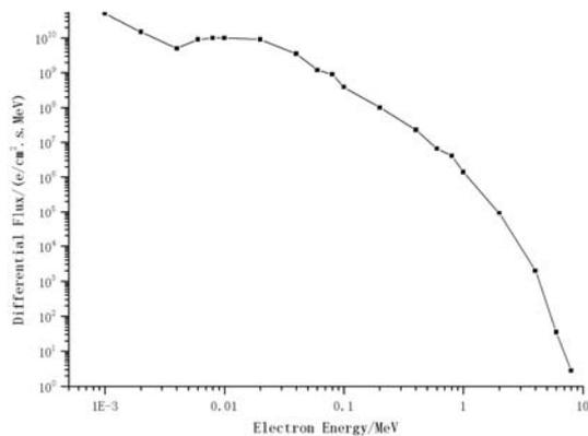
Fig.2 Electron differential flux spectrum in GEO
