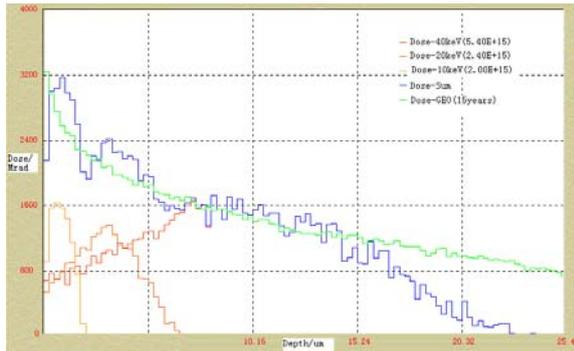
Fig.4 Predicted simulation dose profile and orbital dose profile in GEO
