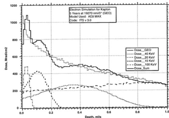
Fig.3 Predicted simulation dose profile and orbital dose profile in GEO
