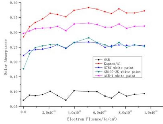
Fig.5 Curve of Degradation datas of five materials
