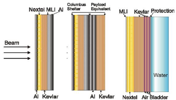
Fig. 7: Schematic configuration layout of: the Columbus target without (left) and with (center) Internal Out-Fitting added; the flexible multi-layer REMSIM target (right).
