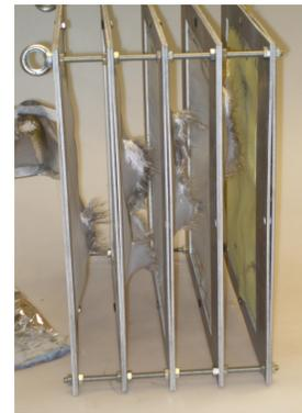
Fig. 5: Light flexible impacted by a 5 mm Al sphere at 7.13 km/s, 45° (EMI test #4914). Test passed with minimal damage to the ballistic restraint.
