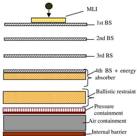
Fig. 4: Typical layout of inflatable structure (REMSIM configuration).
