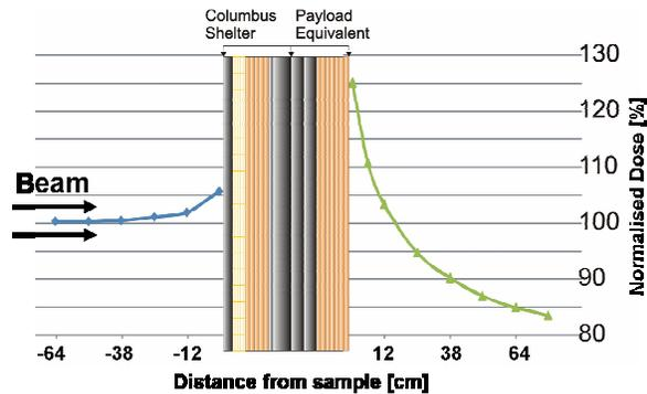
Fig. 10: Relative dose measured as a function of the distance along the proton beam axis for Columbus plus Equipment Equivalent target
