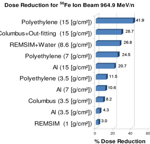
Fig. 9: Dose reduction vs target, obtained irradiating the samples with a  $1 \text{ GeV n}^{-1} {}^{56}\text{Fe}$  ions beam, with reference to the unshielded beam dose
