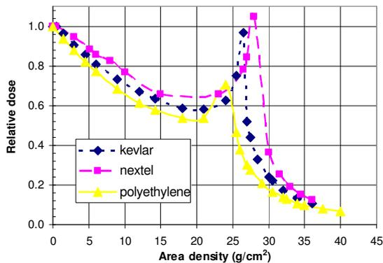
Fig. 8: Bragg curves of  $968 \text{ MeV n}^{-1} {}^{56}\text{Fe}$  -ions measured in HDPE, Kevlar and Nextel. Dose is normalized to the value measured without shielding.
