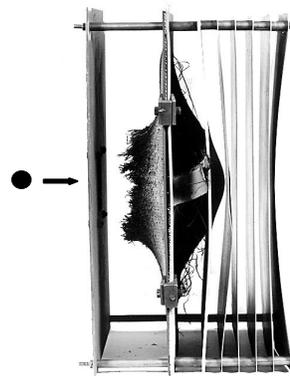
Fig. 2: Columbus SWS target impacted by a 15 mm (5 g) Al sphere at 6.51 km/s (test #8611, failed)
