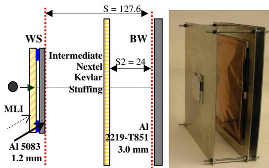
Fig. 3: Layout of the ATV ICC test target (all dimensions in mm) and actual target before test.
