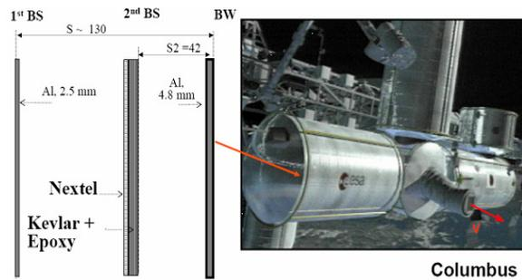
Fig. 1: Layout of the Columbus debris shield configuration
