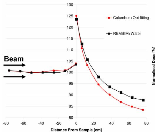
Fig. 11: Relative dose as a function of the distance along the 1 GeV proton axis for the Columbus plus out-fittings and for the REMSIM plus water targets.
