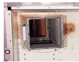
Fig. 2. darkening of a white paint on LDEF
