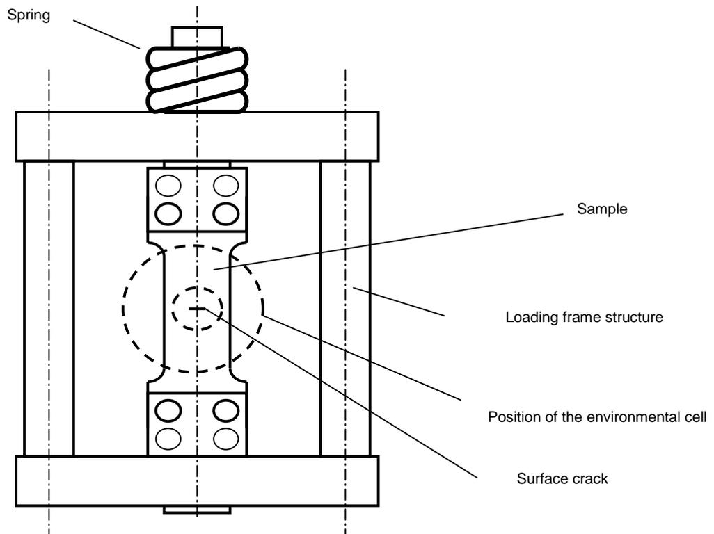
Figure 3. Schematic of the loading frame used to load the samples.
