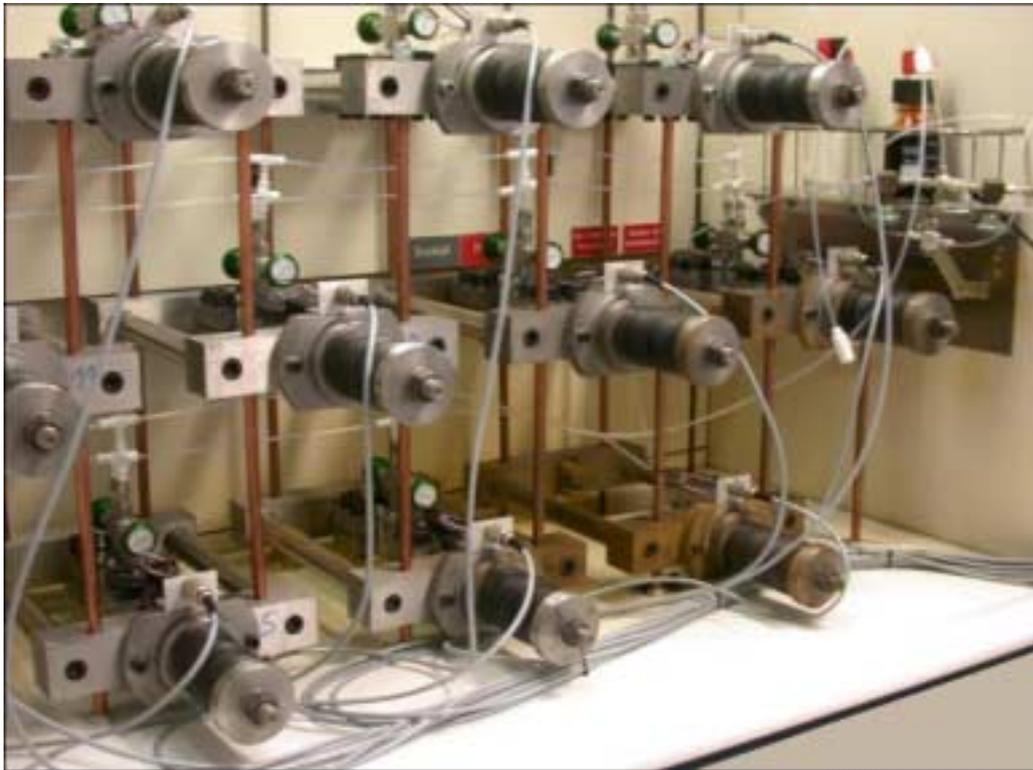
Figure 4. Photo of the SCC test set-up.
