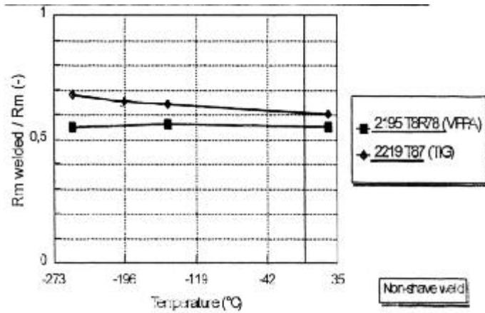
Fig. 4 - Comparison between Al-Li 2195 and conventional Al 2219. Joint coefficient values
