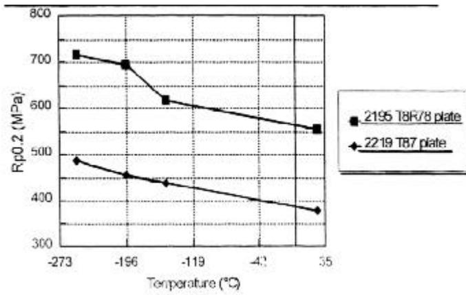
Fig. 2 – Comparison between Al-Li 2195 and conventional Al 2219. Average yield strength values L and T
