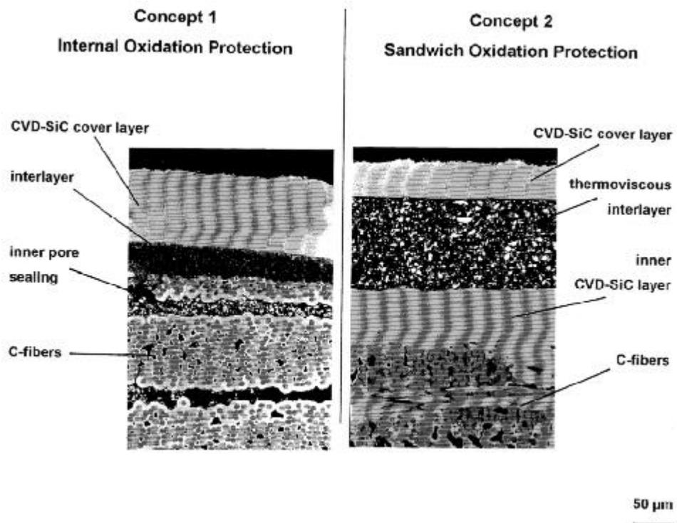
Fig. 7 – Oxidation protection systems developed. The left one was not promising as expected.
