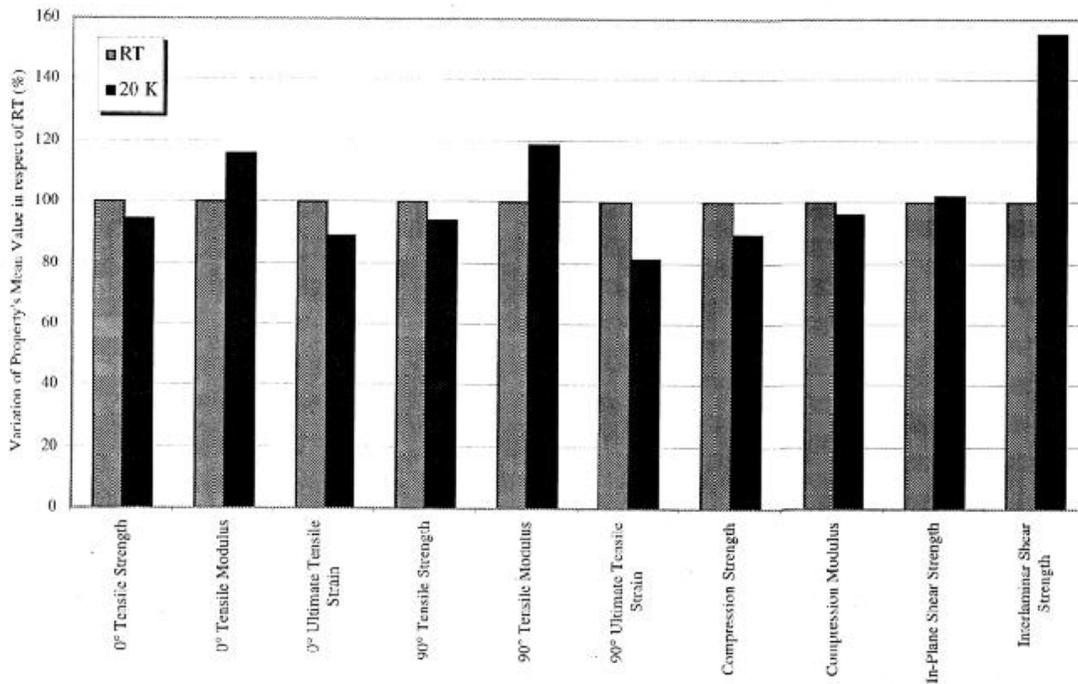
Fig. 5 – CFRP 954-2 / IM 7 UD - Comparison of mechanical properties at 20K and RT
