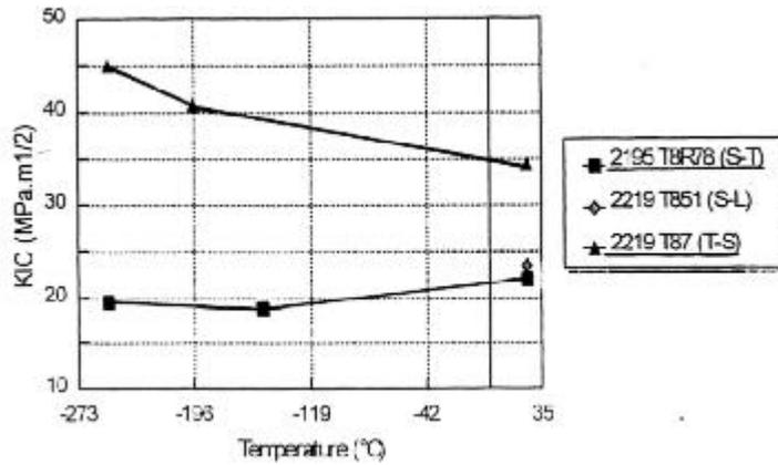
Fig. 3 - Comparison between Al-Li 2195 and conventional Al 2219. Fracture toughness values
