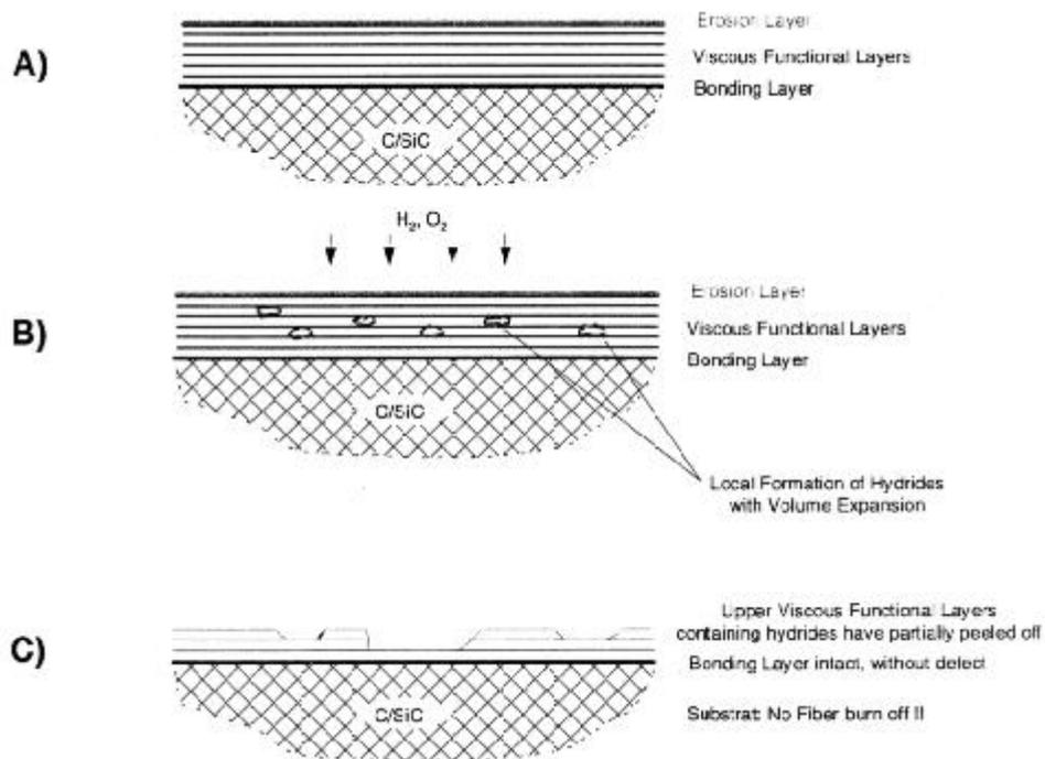
Fig. 8 – Tentative interpretation of the degradation of a multilayers CMC coating.
