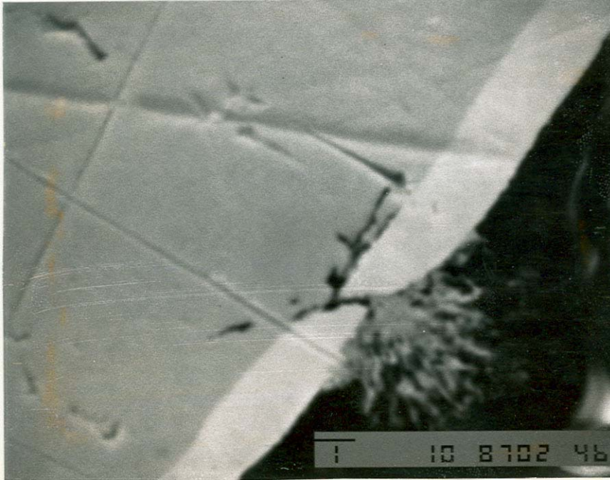
Figure 6: A microsection through a defect in the gold plating. It shows that silver is also attacked under the gold plating.
