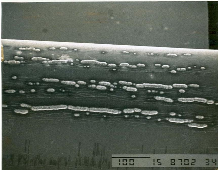
**Figure 5: Gold coated silver is subjected to bending where after it is exposed to atomic oxygen. The horizontal artefacts are oxidised silver through defects in the gold plating.**
