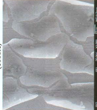
Figure 15 - SEM micrographs of the test panels A17075 after chemical conversion coating treatment with Alodine 5700 at different times of immersion.
