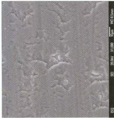
Figure 14 - SEM micrographs of the test panels AI5083 after chemical conversion coating treatments.
