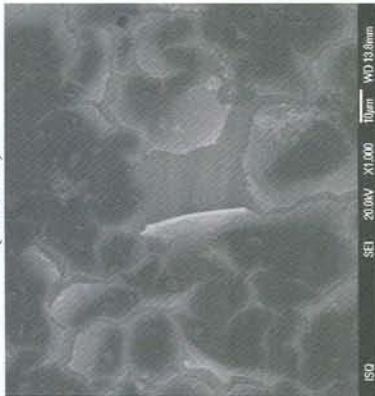
Figure 16 - SEM micrographs of the test panels Al2219 after chemical conversion coating treatment with Alodine 5700 at different immersion times.
