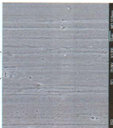
Figure 15 - SEM micrographs of the test panels A17075 after chemical conversion coating treatment with Alodine 5700 at different times of immersion.
