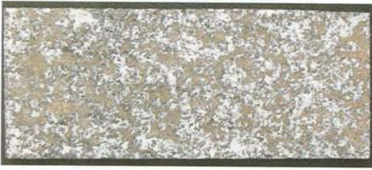
Figure 5 - Illustrative photographs of the 'as received' aluminium alloy test panels after salt spray tests.
