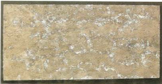
Figure 5 - Illustrative photographs of the 'as received' aluminium alloy test panels after salt spray tests.
