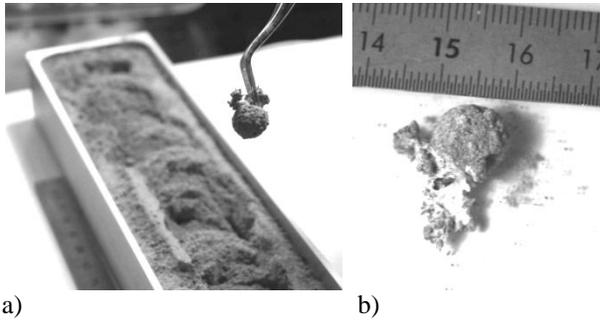
Fig. 8: a) Sample #6 being extracted from the regolith simulatant container after the test. b) Size of sample.
