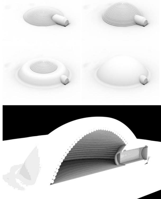
Fig. 2: Building the wall using a temporary inflatable support. Sequence: left to right and top to bottom.
