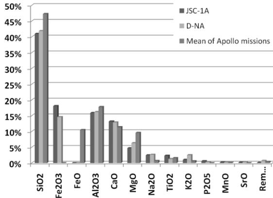
Fig. 4: Comparison of chemical analysis between JSC-1A, D-NA-1, and an average of lunar soil samples from Apollo missions<sup>2</sup>.
