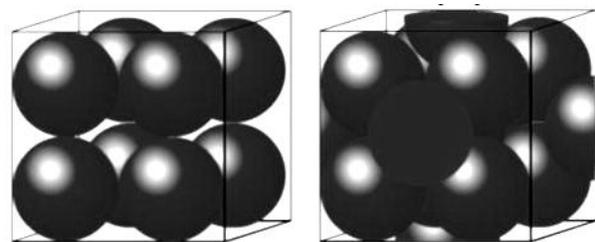
a) Simple Cubic Packing. Void/full ratio = 48%.
