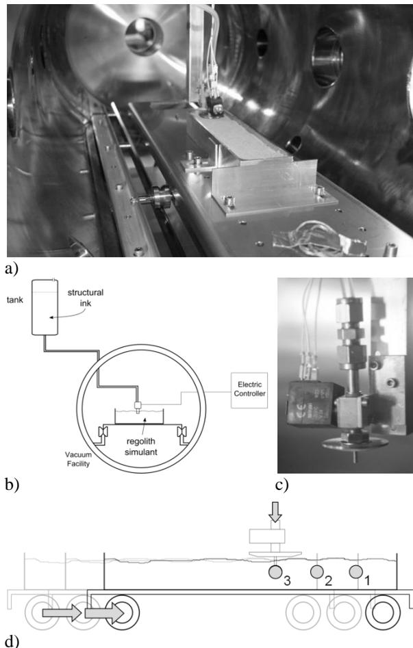
Fig. 7: a) Test setup inside Alta vacuum facility CA-2. b) Schematic layout of the test setup. c) The injector nozzle and valve. d) Injection sequence.
