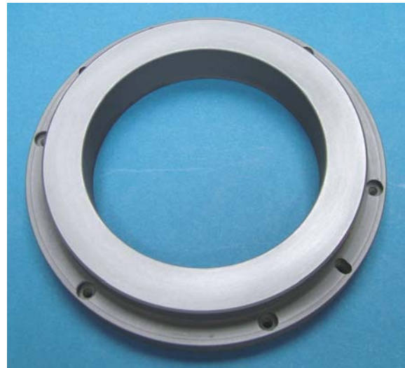
Fig. 10 Keronite + MoS 2 composite coating on EMIR GRISM cryostat wheel bearing currently used for space observation. The coating has been extensively evaluated for wear resistance, debris formation, stick-slip behaviour, ultra-low friction. Courtesy: Instituto de Astrofísica de Canarias
