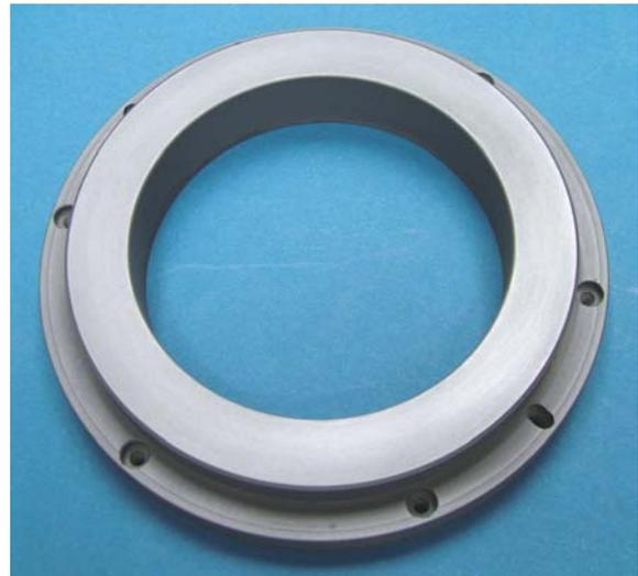
Fig. 10 Keronite + MoS<sub>2</sub> composite coating on EMIR GRISM cryostat wheel bearing currently used for space observation. The coating has been extensively evaluated for wear resistance, debris formation, stick-slip behaviour, ultra-low friction. Courtesy: Instituto de Astrofísica de Canarias
