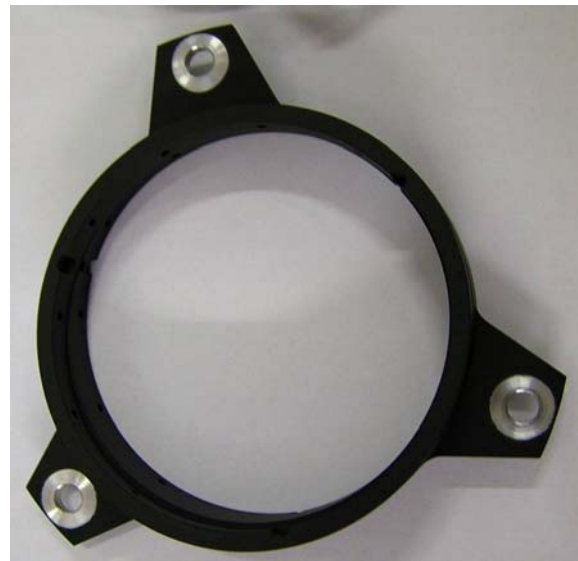
Fig. 11 Barrel for satellites treated with new black Keronite. The black Keronite coating has recently been extensively tested in humidity, vibration, debris formation, low optical reflectivity tests and as a sub-layer for adhesive bonding. Courtesy: Cilas Marseille
