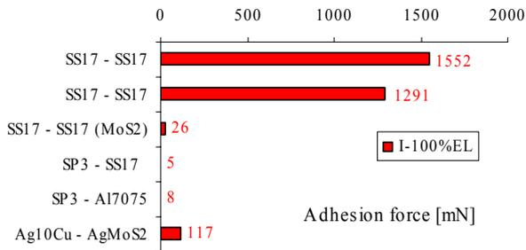
Fig.8 Adhesion force under impact for different combinations with MoS<sub>2</sub>:coatings and composites provide good prevention of cold welding (SP3 = Vespel SP3, Ag10Cu = coin silver, AgMoS<sub>2</sub> = silver composite with 15% MoS<sub>2</sub>).
