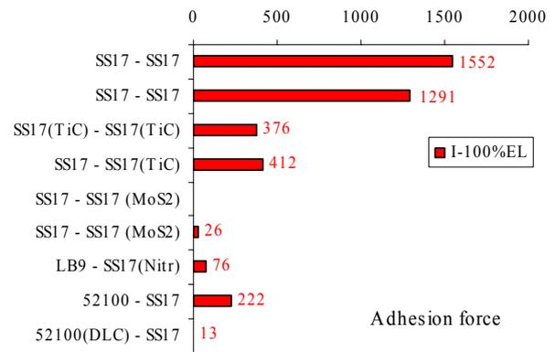
Fig.6 Adhesion force as function of static load for different coatings on steel: lowest adhesion for SS17-7PH (SS17) with MoS<sub>2</sub>. Higher adhesion for TiC (coatings was broken). Negligible adhesion between bronze (LB9) and SS17-7PH (LB9-SS17(Nitr)). Low adhesion between AISI52100 and SS17-7PH, can further be decreased by use of DLC coating (“52100(DLC)-SS17”).
