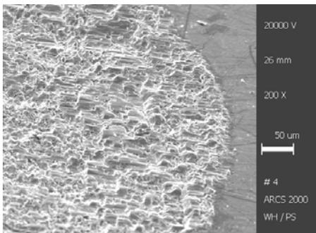
Fig. 14 Surface of disc SS17-7ph with MoS<sub>2</sub> coating after fretting tests (compare to Fig. 11 for adhesion forces): lubrication effect was lost after less than 200 second fretting movement (confirmed by EDAX-mapping: no Mo present in contact area).
