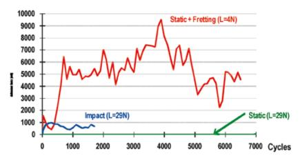
Fig. 2. Adhesion force as a function of the number of cycles (one closing and separation each) [8]. Comparison of adhesion under static (load 29 N), impact (load 29 N) and fretting (load 4 N) conditions under vacuum. The risk and severity of adhesion increase with contact in the order static, impact, fretting (maximum adhesion: static  $0.1 \, \text{N}$  after >25000 cycles; impact  $0.96 \, \text{N}$ ; and fretting  $9.5 \, \text{N}$ ).
