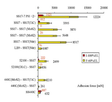
Fig. 11. Adhesion force of steel-based coatings under impact (I) and fretting (F) conditions. Coatings in general reduce adhesion. For SS17-7PH, no tested coating of the disc is able to reduce adhesion significantly (TiC,  $MoS_2$  or nitriding). In contacts between AISI 440C and SS17-7PH, TiC should be avoided. The efficiency of grease (Braycote 601) is not significant in AISI 440C in contact with itself, and that of the  $MoS_2$  coating under fretting is limited to low endurance
