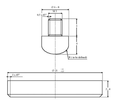
Specimen for static, impact, fretting tests
