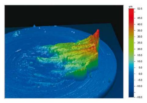
Fig. A.3. Example of a ball after a friction test.
