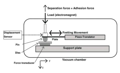
Fig. B.1. Functional sketch of a fretting device.
