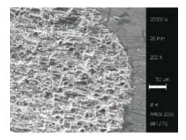
Fig. 15. Surface of disc of SS17-7PH with MoS<sub>2</sub> coating after fretting tests (compare with Fig. 11 for adhesion forces). The lubrication effect was lost after fretting movements lasting less than 20 s (confirmed by EDAX mapping; no Mo was present in the contact area).
