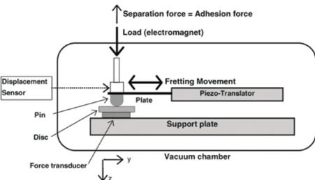
Fig. A.2. Fretting facility: device (top left); inside view (top right); functional sketch (bottom).
