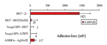
Fig. 9. Adhesion force under impact for different combinations with  $MoS_2$ . Coatings and composites are effective in preventing cold welding (SP3 = Vespel SP3, Ag10Cu = coin silver, AgMoS<sub>2</sub> = silver composite with 15 vol%  $MoS_2$ ).
