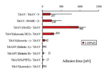
Fig. 8. Adhesion force under impact for different coatings on Ti alloys. Hard coatings provide good protection against cold welding, but solid lubricants (MoS<sub>2</sub>, WS<sub>2</sub>) fail.
