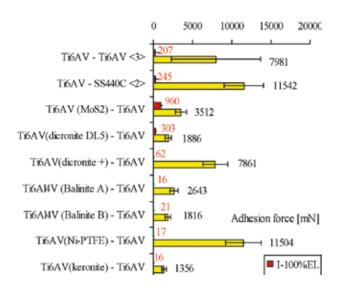
Fig. 13. Adhesion force of coatings on Ti6AV under impact (I) and fretting (F) conditions. Under impact, hard coatings prevented cold welding, but under fretting, all coatings were broken. The lowest adhesion forces were found for Ti6AV with thin (~6 μm) coatings of Balinite B and Keronite.
