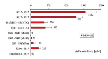
Fig. 6. Adhesion force as a function of static load for different coatings on steel. The lowest adhesion is for SS17-7PH (SS17) with MoS<sub>2</sub>, The adhesion is highest for TiC (coatings were broken), and negligible between bronze (LB9) and SS17-7PH (LB9-SS17(Nitr)). The low adhesion between AISI 52100 and SS17-7PH can be further reduced by using a DLC coating ('52100(DLC)-SS17').
