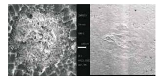
Fig. 16. Comparison of Al coatings under fretting. *Left*: The hard anodising on Al7075 was broken. *Right*: The Keronite coating on Al AA 2219 shows no fretting marks (compare with Fig. 11 for adhesion forces).
