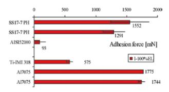
Fig. 4. Adhesion force under impact for materials in contact with themselves. The highest adhesion forces are found for stainless steels with nickel (e.g. SS17-7PH) and Al alloys (Al AA7075), medium for Ti alloy, and the lowest for bearing steel AISI 52100 (no Ni).
