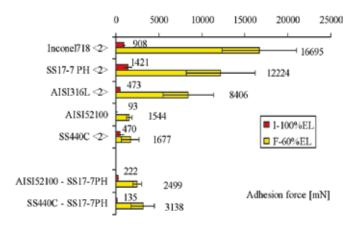
Fig. 10. Comparison of adhesion force under impact (I) and fretting (F) for different steels and Ni alloys in contact with themselves. Fretting initiates higher adhesion, but for ferrous alloys adhesion decreases with decreasing Ni content, as indicated in [10].
