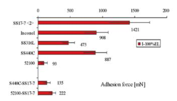
Fig. 5. Adhesion force under impact for different types of steel in contact with themselves: austenitic steels and Ni seem to promote high adhesion: SS17-7PH (7% Ni), AISI 316L (11% Ni) and Inconel 718 (52% Ni). No adhesion was found for AISI 52100 in contact with itself ('52100'). The high adhesion of AISI 440C has yet to be confirmed. With combinations of different steels, adhesion seems to increase in those in contact with steels with a higher tendency to cold welding (indicated by arrows).
