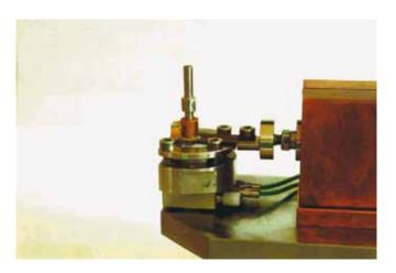
Fig. 3. Detail of the fretting device, showing the fixation of the pin (upper rod) and the disc (mounted directly on a force transducer). The piezo actuator that generates the fretting movement can be seen on the right.
