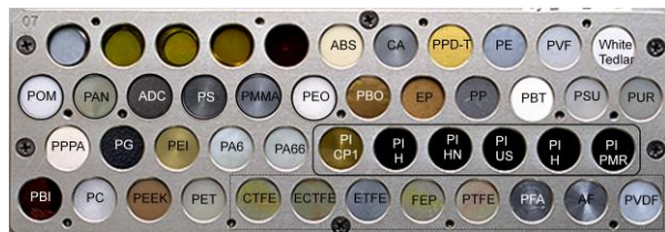
Fig. 1. Photograph of MISSE 2 PEACE Polymer experiment tray before exposure
