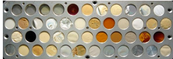
Fig. 2. Photograph of MISSE 2 PEACE Polymer experiment tray after exposure
