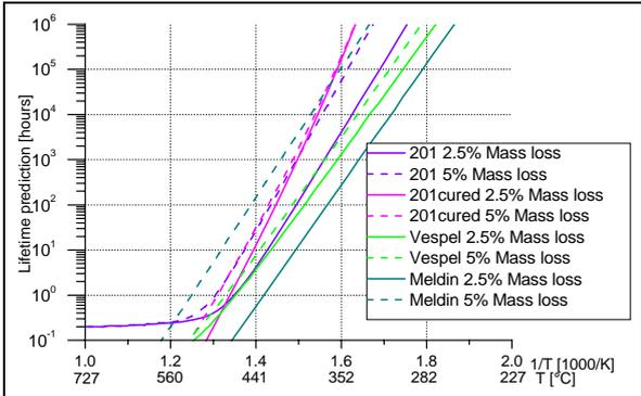
Fig 2. Comparison of lifetime prediction of the studied polyimide materials at 2.5% and 5% mass loss
