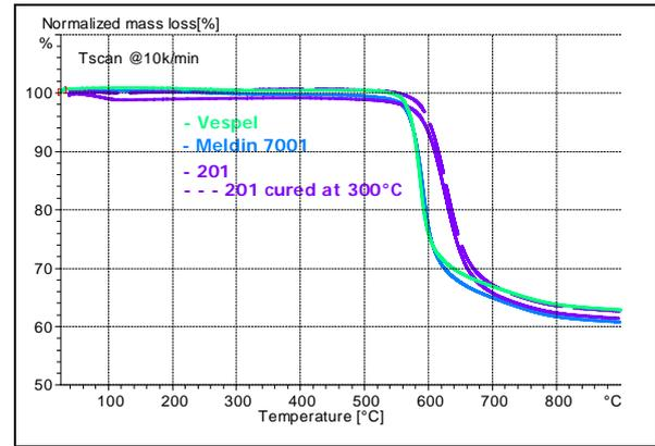
Fig.1 Comparison of normalized tscan curves at 10 °C/min of polyimide materials
