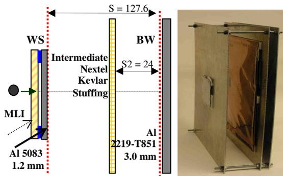
Fig. 3: Layout of the ATV ICC test target (all dimensions in mm) and actual target before test.
