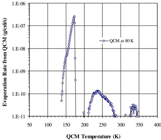
Fig. 6: QCM thermogravimetric analysis on Kevlar KM2 CS705 WR at 45°C.
