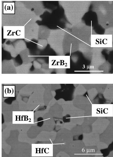
Fig. 4. SEM back-scattered micrographs of dense SPSed ZZS (a), and HHS (b) products.
