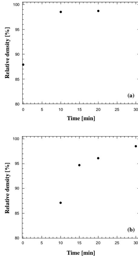
Fig. 3. Effect of SPS time on relative density of sintered ZZZS (a), and HHS (b) powders synthesized by SHS ( $T_D=1800\text{ }^\circ\text{C}$ ,  $t_H=10\text{ min}$ ,  $P=20\text{ MPa}$ ).
