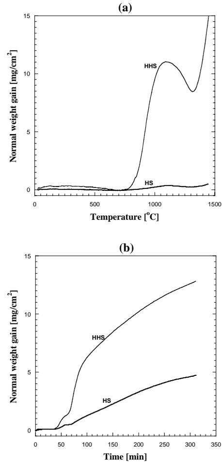
Fig. 5. Specific weight change during TGA oxidation in air of the sintered HS and HHS samples as a function of (a) temperature (non-isothermal run with the heating rate equal to 2 °C/min) and (b) time (isothermal run at 1450 °C).
