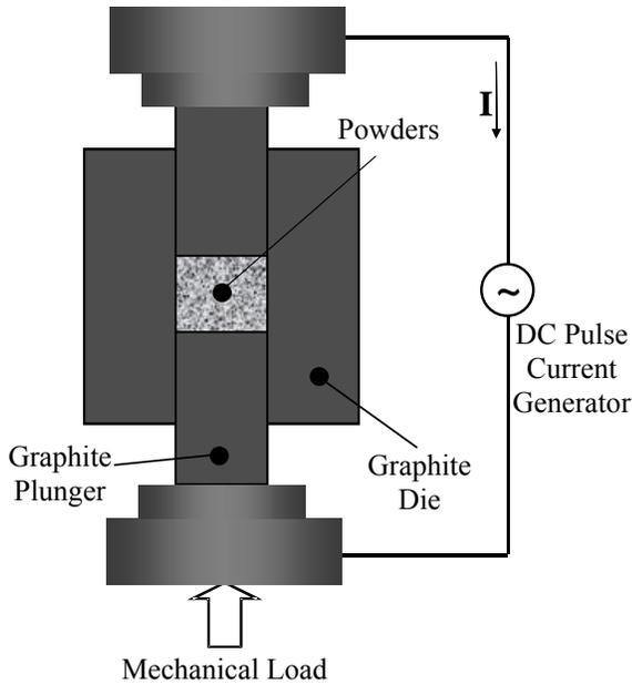
Fig. 1. Schematic representation of the Spark Plasma Sintering (SPS) system.
