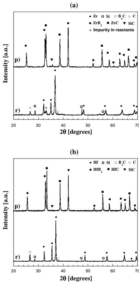
Fig. 2. Comparison of XRD patterns of r) starting reactants and p) products obtained by self-propagating high-temperature synthesis according to reaction (2): (a) ZZZS, and (b) HHS.
