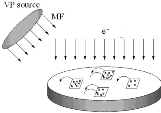
Fig. 2. Scheme of experiments on studying combined action of molecular flux and electron radiation on quartz glass samples
