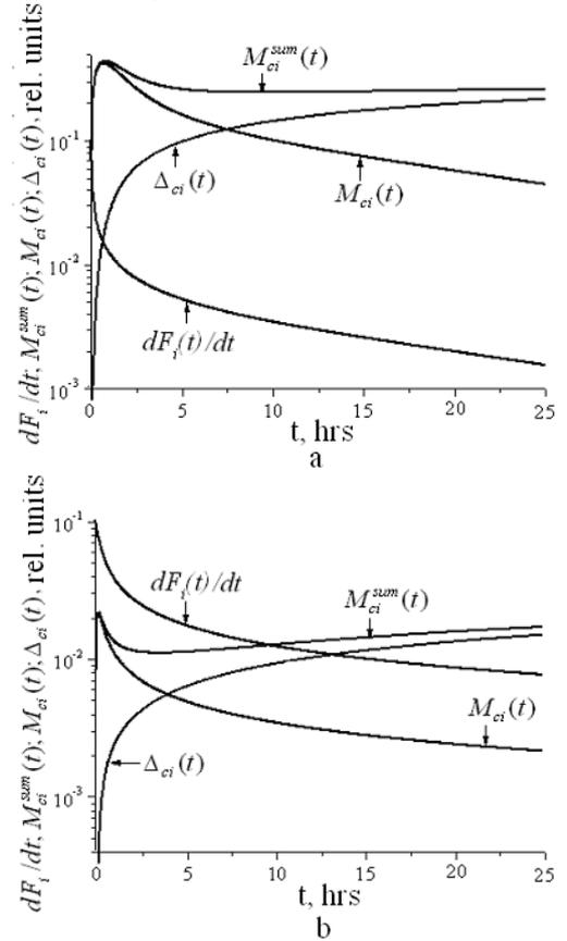
Fig. 4. Time dependences of basic functions defining VP accumulation on substrate surfaces at different temperatures: a – T= 40°C; b – T= 60°C
