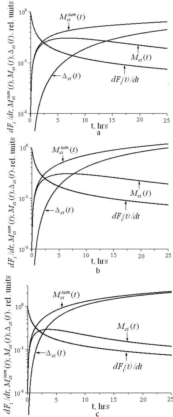
Fig. 5. Time dependences of basic functions defining VP accumulation on substrate surfaces: *a* – without irradiation; *b* – if considering (4); *c* – for constant parameter  $\chi_{ci}^{rad} = \beta\chi_{ci}$
