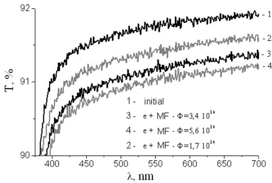
Fig. 3. Spectral transmittances of quartz glass samples after action of MF and different electron fluxes ( $cm^{-2}$ ): 1 –  $\Phi=0$ ; 2 –  $\Phi=1.7 \times 10^{14}$ ; 3 –  $\Phi=3.4 \times 10^{14}$ ; 4 –  $\Phi=5.6 \times 10^{14}$
