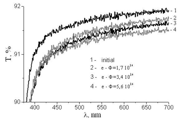
Fig. 1. Spectral transmittances of quartz glass samples irradiated by different electron fluxes ( $cm^{-2}$ ): 1 –  $\Phi=0$ ; 2 –  $\Phi=1.7 \times 10^{14}$ ; 3 –  $\Phi=3.4 \times 10^{14}$ ; 4 –  $\Phi=5.6 \times 10^{14}$
